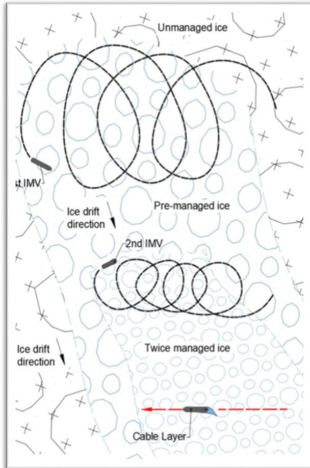
Figure 4b. Ice Management for drifting ice from other directions than ahead.
